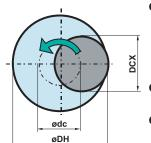
● How to calculate the theoretical center of the tool path.
